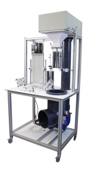
The aerodynamics bench is designed to perform a variety of experiences in the field of fluid mechanics, using a controlled airstream for it.
